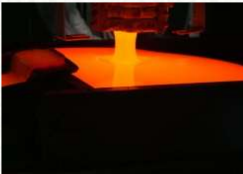
Pouring of melt into pre - heated mould
