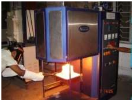
Raising hearth furnace
